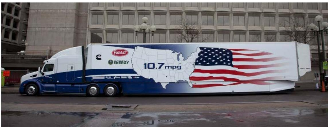
**Figure 6: SuperTruck program technology - Class 8 truck that accomplishes 10 mpg**
